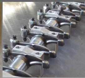
The team has designed a new type of rocker pedestals. Istvan Popovics has manufactured them in aircraft spec aluminium for the team. They are much stronger than original items and 1/3 of the weight compared to the steel-pedestals offered by other Healey specialists.
