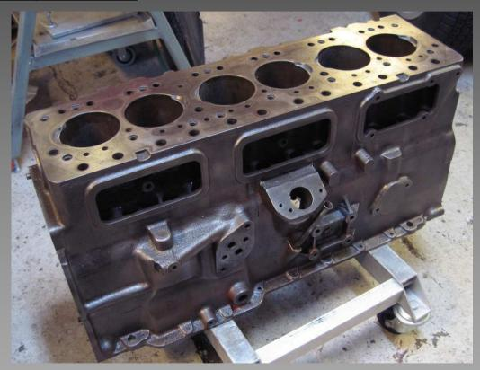
The new engine block ready for machining.
