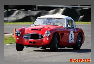
Finally after years of investigation the Healey 3000 has landed historically and settled in the GT class -65. This means that we may replace the 4,5" 72 spoke wire wheels with lighter, stronger and wider 6" minilites.
